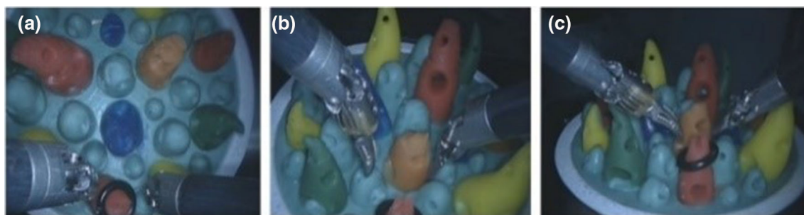
Fig. 11 User studies for the hand–eye coordination. a \vartheta = 10^\circ \pm 5^\circ ; b \vartheta = 40^\circ \pm 5^\circ ; c \vartheta = 70^\circ \pm 5^\circ
