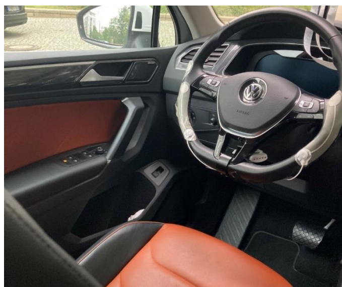
Figure 2. Recording system with the ECG electrodes in the research car.
