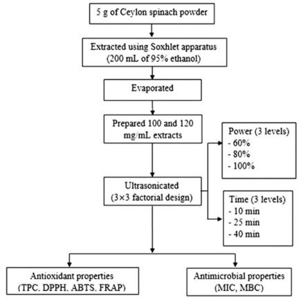
Figure 1. Design of the ultrasonic experiment.
