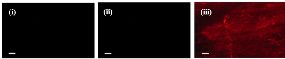
Figure 5. Fluorescent images of fibrous scaffolds made of E0500 immunostained for fibronectin (red). (i) Scaffolds were incubated in culture medium without cells for 28 days and were decellularized (−C/+D). Negative staining indicates the absence of fibronectin in the scaffolds; (ii) scaffolds were cultured with NIH3T3 cells for 28 days and decellularized (+C/+D) but were not immunostained for fibronectin (negative control); and (iii) scaffolds were cultured with NIH3T3 cells for 28 days and decellularized (+C/+D), followed by immunostaining for fibronectin. The positive staining in (iii) indicates the presence of cell-derived fibronectin on the scaffolds. Scale bars are 10 μm.
