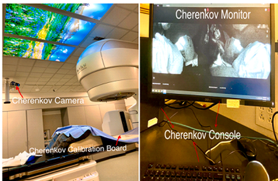
Fig. 1. The Cherenkov imaging system commissioned for clinical use in our hospital. The left panel shows a Cherenkov camera mounted to the right of the treatment couch. The Right panel shows the Cherenkov image display at the treatment console.
