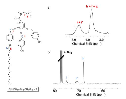
**Figure 14.** Zooms of the NMR spectra of the polyoxazoline derived from TAPOx: (**a**) <sup>1</sup>H NMR spectrum between 2.5 and 5.5 ppm (signals labelled in red); and (**b**) <sup>13</sup>C NMR spectrum between 50 and 80 ppm (signals labelled in blue).
