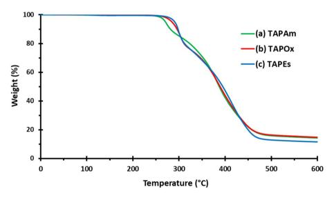
**Figure 13.** TGA thermogram of (**a**) TAPAm, (**b**) TAPOx and (**c**) TAPEs recorded at a heating rate of 10 °C/min in nitrogen atmosphere.
