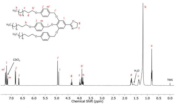
Figure 6. <sup>1</sup>H NMR spectrum in CDCl<sub>3</sub> of TAPOx.
