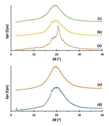
Figure 10. XRD patterns of TAPAm recorded on heating at: (a) 70  $^{\circ}$ C, (b) 90  $^{\circ}$ C and (c) 110  $^{\circ}$ C on first heating; and (d) 80  $^{\circ}$ C and (e) 110  $^{\circ}$ C on second heating.
