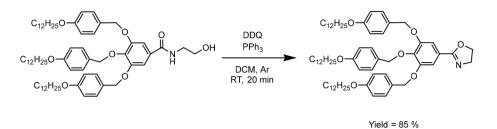
Figure 5. Synthesis of 2-(3,4,5-tris(4-dodecyloxybenzyloxy)phenyl)-2-oxazoline (TAPOx).
