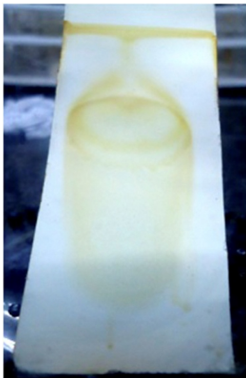
Fig. 1. TLC silica gel 60 (5 × 7.5 cm Merck, Germany), Aluminum backed showed single band from partially purified active molecule found at top of the gel. The rings found in middle of the gel show the running downstream to upstream.
