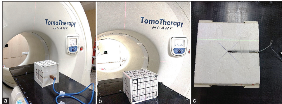
Figure 2: Setup of detector in a virtual water phantom for the measurement of beam quality (a) Ionization chamber (b) side view for the diode (c) bottom of the phantom for the diode
