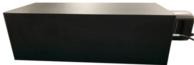
Figure 3. A photograph of the prototype solid spectrometer constructed in accordance with the proposed design with dimensions of 570 (length)x270 (width)x180 (height) mm, not including the BSI-CMOS camera.
