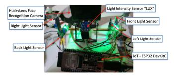
Figure 7. Guidance Landing System (GLS) hardware components.
