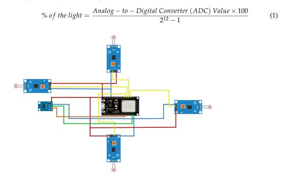
Figure 8. Part of Guidance Landing System (GLS) circuit connections diagram.
