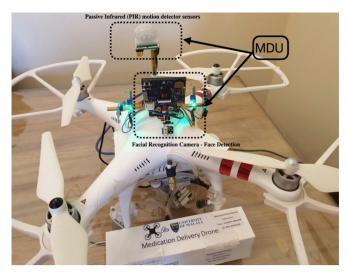
Figure 6. Guidance Landing System (GLS) and Motion Detection Unit (MDU).
