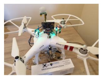
Figure 1. Drone with facial recognition and medical delivery box.
