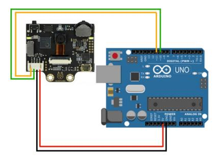
Figure 4. Circuit connections diagram for the Huskylens facial recognition camera.
