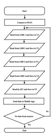
**Figure 9.** Flowchart of Guidance Landing System. Notes: LDR—Light-Dependent Resistor; V1, V2, V3, V4, and V5 are the virtual pins in the IoT mobile apps.
