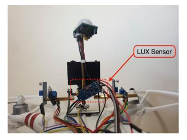
**Figure 12.** The sensor (Lux) was moved to the backside of the drone to detect the light from the controlled source.
