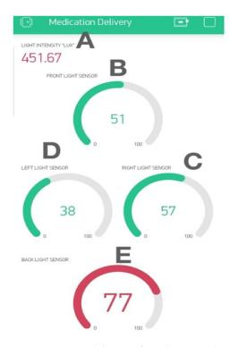
**Figure 13.** IoT mobile app of Guidance Landing System (GLS). (**A**) The upper numerical value shows the light intensity the backside. (**B**) The light intensity percentage of the front-side sensor. (**C**) Light intensity percentage of the right-side sensor. (**D**) Light intensity percentage of the left-side sensor. (**E**) Light intensity percentage of the back-side sensor.
