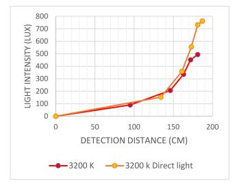
**Figure 16.** Graph shows the relation between light intensity (Lux) and detection distance (cm) for 3200 K soft light and 3200 K direct light without diffuser.
