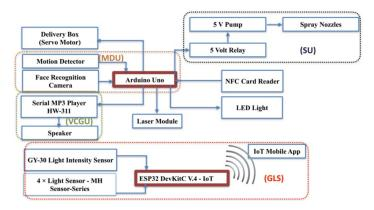
Figure 5. Medical delivery drone enhanced components for Guidance Landing System.
