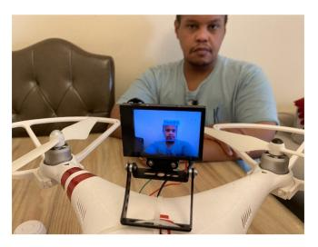
Figure 2. Facial recognition to identify specific user on the medical delivery drone.
