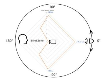
**Figure 14.** Compare the required light intensity (Lux) for facial recognition of 3200 K light source without diffuser from front, right, and left side for a fixed distance of detection of 130 cm.
