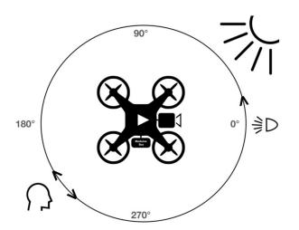
Figure 3. Drone rotates (yaw) 360° around vertical axis at the same location.
