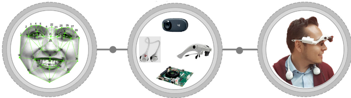
Figure 1. Processes for the development of the face recognition system for people with visual disabilities, (a) face recognition under different facial expressions, (b) implement the devices and adapt them to people with disabilities, (c) system integration.
