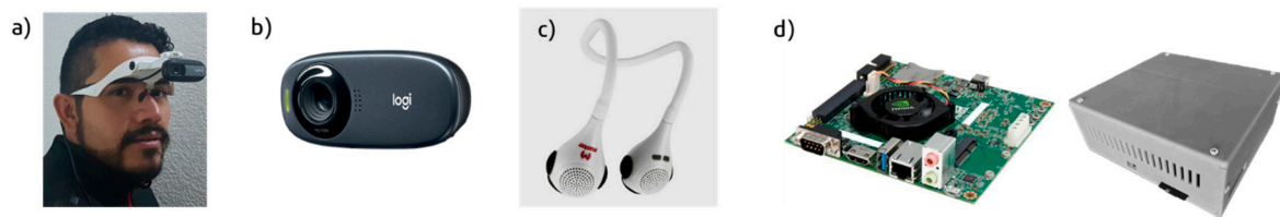
Figure 17. Devices that integrate the face recognition system for people with disabilities. (a) Headband-shaped structure, (b) webcam Logitech c310, (c) sports speakers brand master model MS-SPORTSPK, (d) NVIDIA Jetson TK1 developer kit with 3D printed case.
