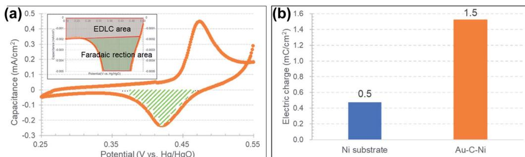
**Fig. 11** (a) Procedure to estimate the component of the faradaic reaction. (b) Comparison of the faradaic reaction component of the stored charge estimated for the Au-C-Ni sample and for the as-received Ni foil.
