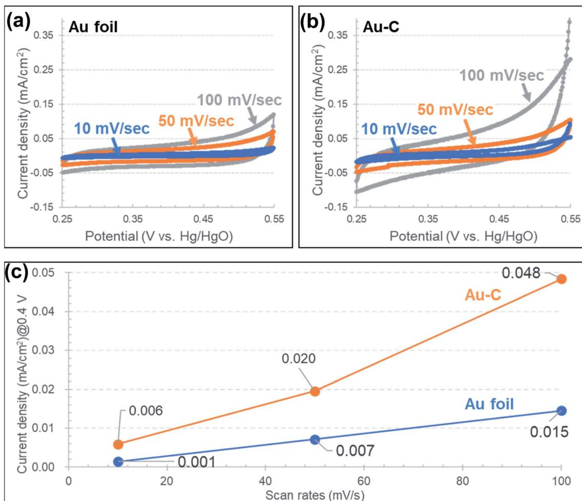
Fig. 7 (a), (b) Typical cyclic voltammograms at scan rates of 10, 50 and 100 mV s<sup>-1</sup> for the samples of as-received Au foil and Au-C, respectively. (c) Scan rate dependence of the capacitance determined at 0.4 V in the cyclic voltammograms (a) and (b).
