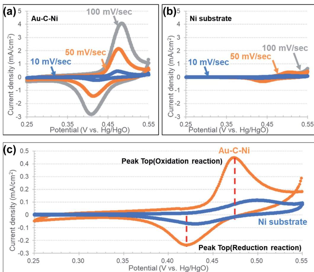
Fig. 8 (a), (b) Typical cyclic voltammograms at scan rates of 10, 50 and 100  $mV s^{-1}$  for the samples of Au-C-Ni and as-received Ni foil, respectively. (c) Comparison of the CV profiles with an enlarged vertical scale for Au-C-Ni and as-received Ni foil at the scan rate of 10  $mV s^{-1}$  shown in (a) and (b), respectively.
