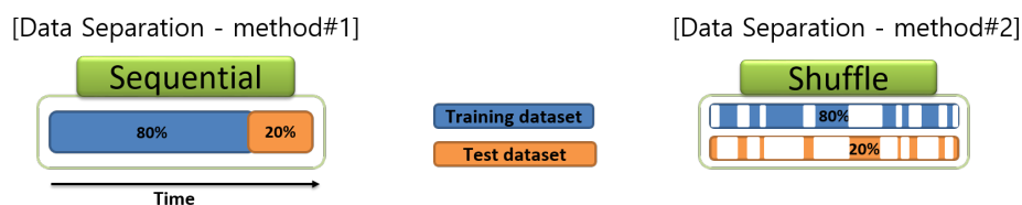
Figure 5. Default data separation methods for the training dataset and test dataset. 20% of the training dataset is used for the validation dataset to prevent the over-fitting calibration model. A shuffled method is controlled by a fixed random seed to compare the performance between calibration algorithms.
