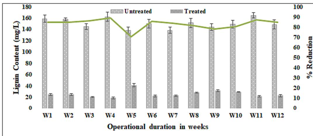
Fig. 6. Reduction in lignin contents in the effluent during 12 weeks of operation through IVFCW.
