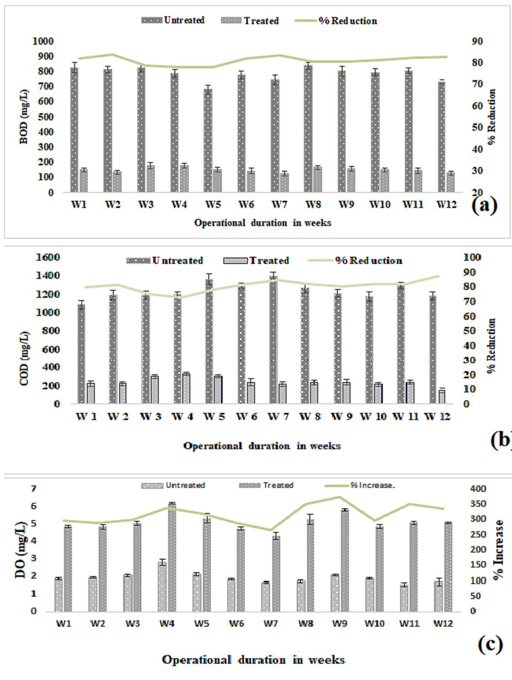
Fig. 4. Comparative variations in BOD<sub>5</sub> (a), COD (b), and DO (c) during 12 weeks of operation through IVFCW planted with *Typha latifolia*.
