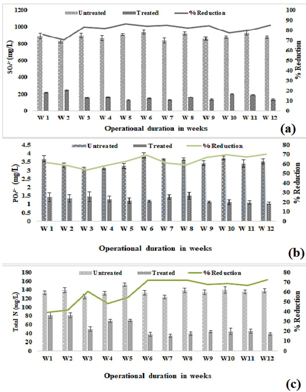
Fig. 5. Comparative variations in sulfates ( $SO_4^{2-}$ ) (a), phosphates ( $PO_4^{3-}$ ) (b), and nitrates ( $NO_3^-$ ) (c) during 12 weeks of operation through IVFCW planted with *Typha latifolia*.
