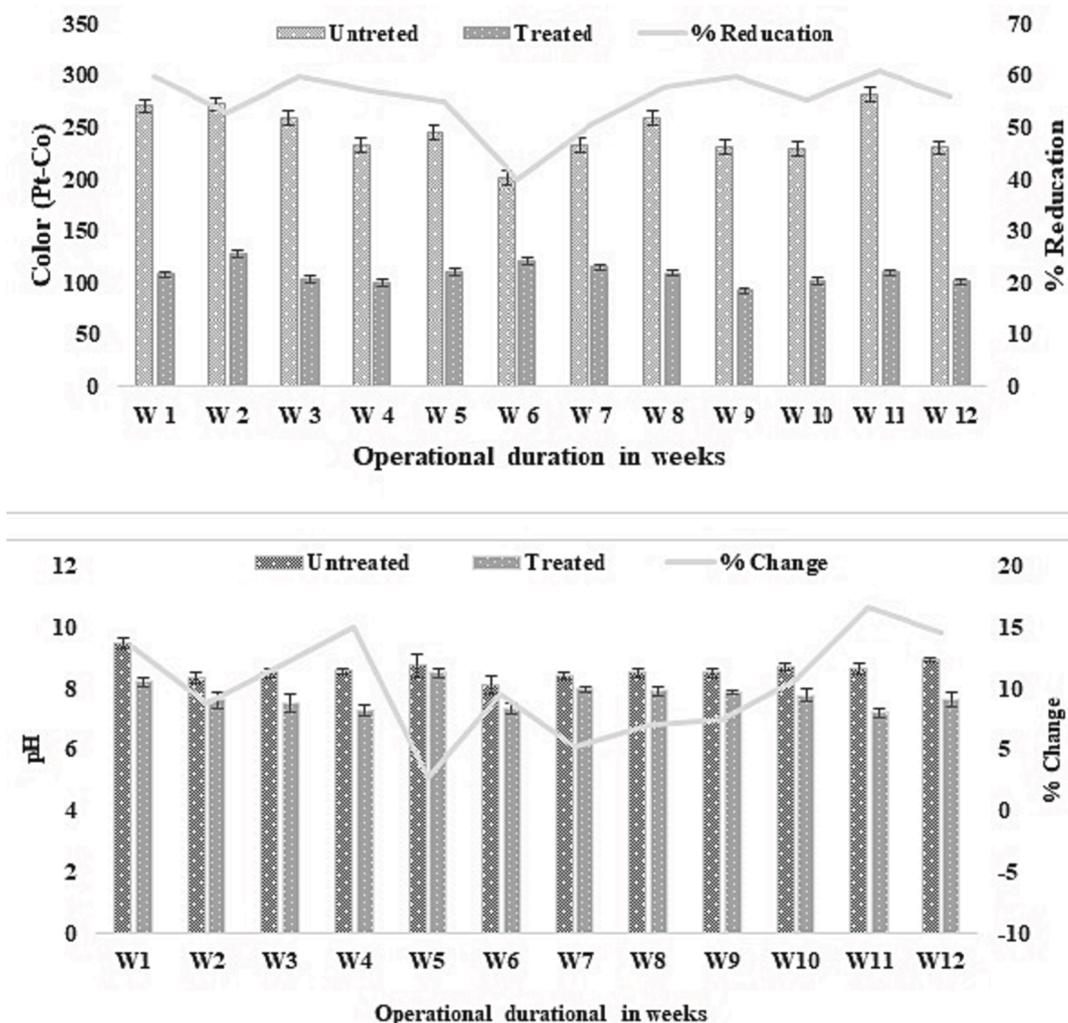
Fig. 2. Color reduction (a) and pH variationin (b) the influent and effluent during 12 weeks of operation through vertical flow constructed wetland (IVFCW)planted with *Typha*.
