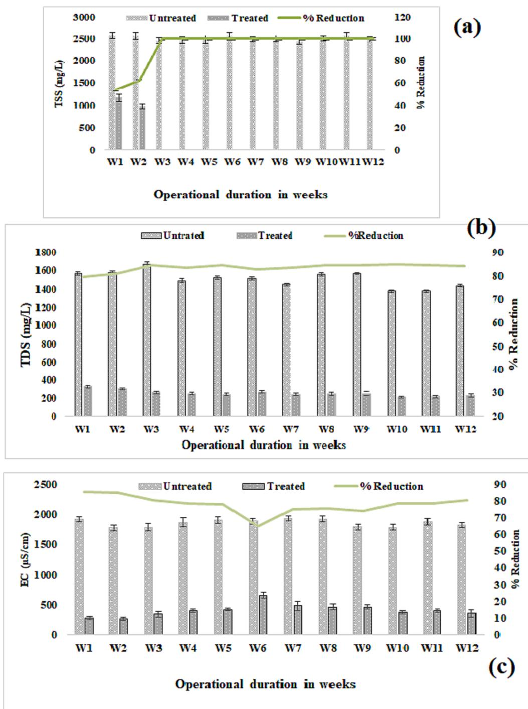
Fig. 3. Comparative variations in TSS (a), TDS (b) and EC (c) influent and effluent during 12 weeks of operation through vertical flow constructed wetland (VFCW) planted with *Typha latifolia*.
