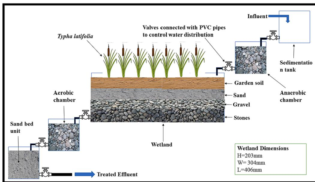
Fig. 1. Schematic illustration of vertical flow constructed wetland (VFCW) planted with *Typha latifolia*.
