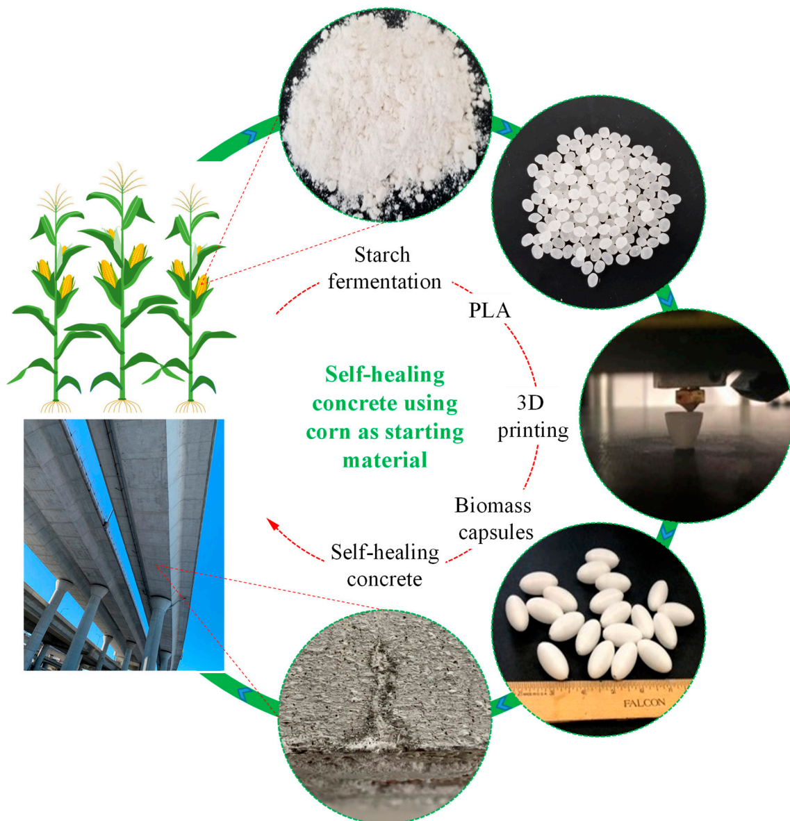
Figure 1. Schematic diagram of self-healing concrete using biodegradable corn as starting material.
