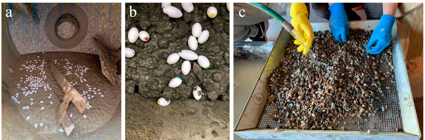
Figure 2. Survivability test procedure: (a) and (b) mixing, and (c) washing and capsule separation.
