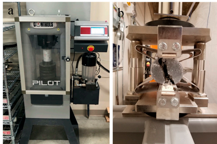
Figure 3. Setup for (a) compression, and (b) split tensile test.
