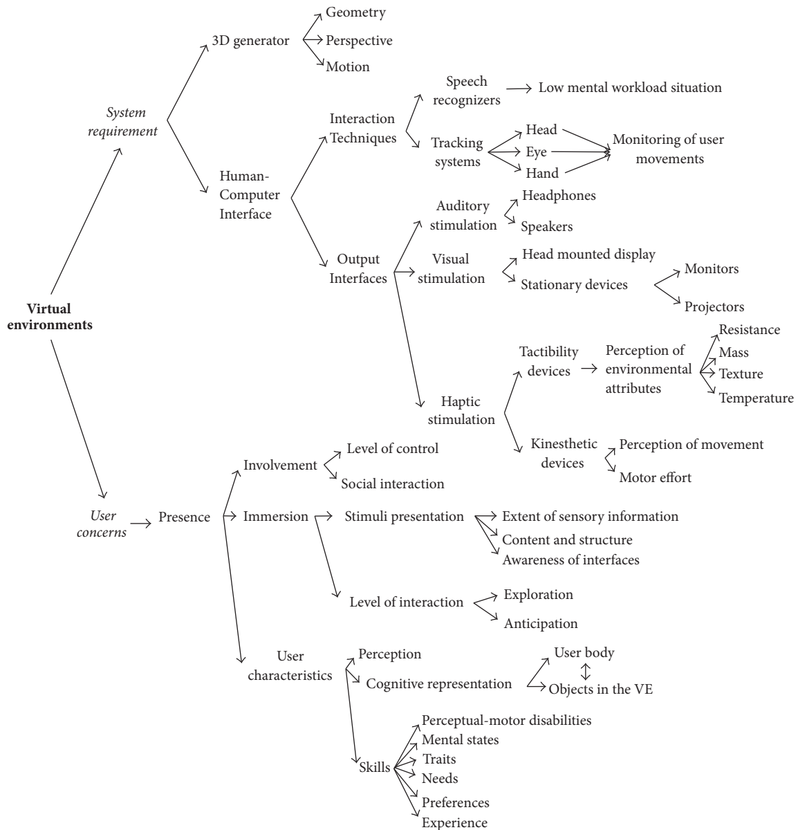
FIGURE 1: Structure of a virtual environment on the basis of two key elements: system requirements and user concerns.
