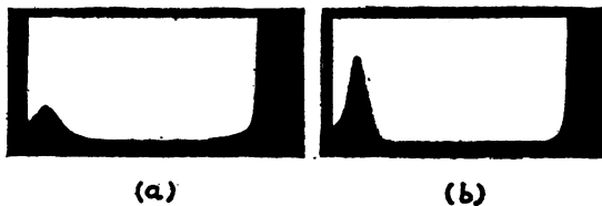
FIG. 3. Sedimentation diagram of 1% solutions of fraction AP-2; (a) before Sevag treatment; (b) after Sevag treatment. Phosphate buffer pH 8, I = 0.1 + 0.15M NaCl. Exposures taken 40 min. after reaching full speed, 60,000 r.p.m. (240,000 g).
