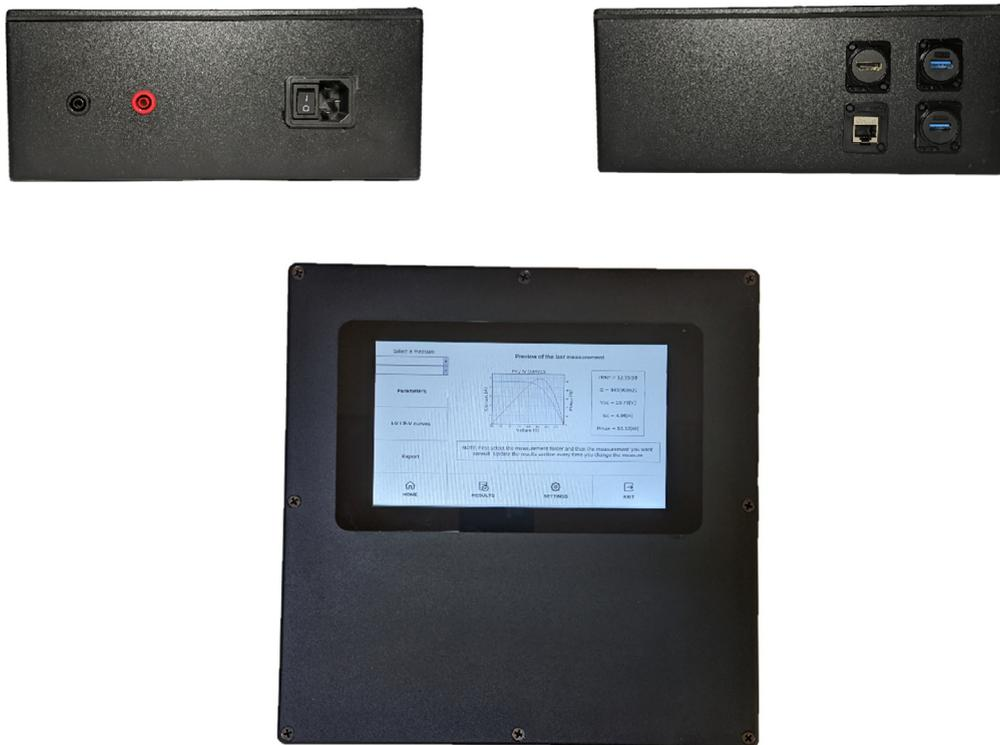
Fig. 9. View of the rear face (I), where there are the positive and negative connectors for the solar panels, and the connector for the electrical network; the front face (II), where are the USB, HDMI, and Ethernet Raspberry Pi connectors of the; and the upper cover (III), which only contains the touch screen.
