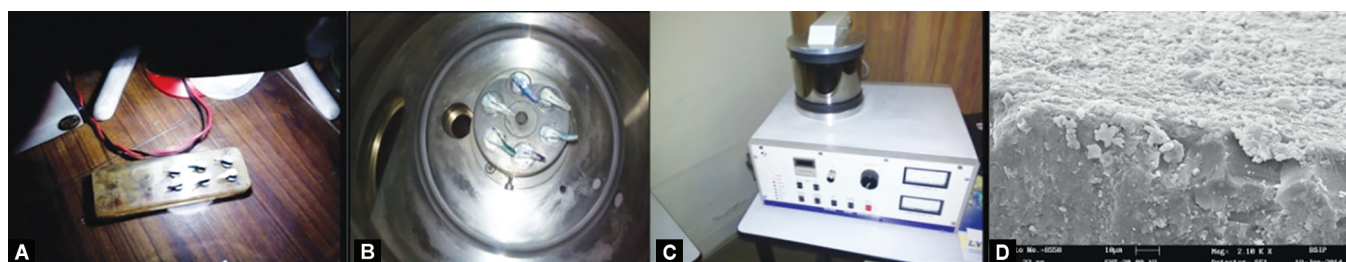
Figs 4A to D: (A) Section tooth mounting; (B and C) Gold spluttering; (D) Scanning electron microscope image of resin tag
