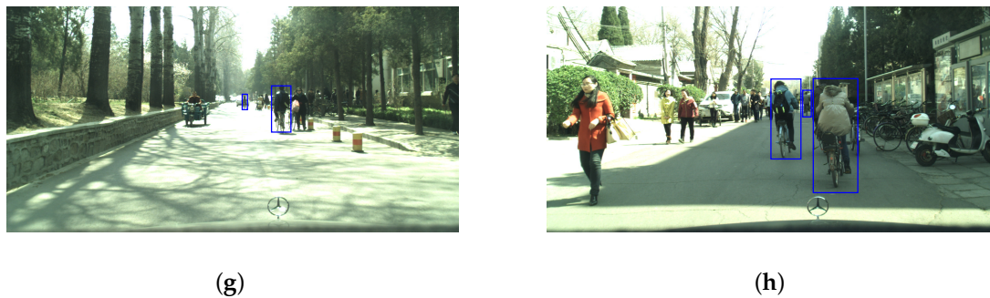
Figure 8. Some results of performing our detector on “Tsinghua-Daimler Cyclist Benchmark” with different scenarios. The images from (a) to (h) are the detection results in complex environments. In order to have a better visual effect, the contrast and brightness of the images above are enhanced for display. Blue bounding boxes represent detected cyclists.
