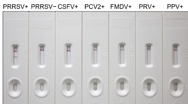
Fig. 4. Specificity of the immunochromatographic strip test. Positive sera of porcine reproductive and respiratory syndrome virus (PRRSV), porcine circovirus-1 (PCV-1), pseudorabies virus (PRV), classical swine fever virus (CSFV), porcine parvovirus (PPV), porcine circovirus-2 (PCV-2), and PRRSV-negative sera were tested by using the immunochromatographic strip at the same time. Result positivity can be decided by visual judgment.
