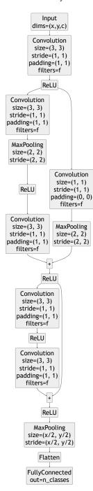
Figure 4. ResNet model architecture.
