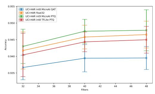
**Figure A1.** Accuracy vs. filters for baseline (*float32*), 8-bit Post-Training Quantization from Tensor-Flow Lite (*int8 TFLite PTQ*), 8-bit Quantization-Aware Training from our framework (*int8 MicroAI QAT*), and 9-bit Post-Training Quantization from our framework (*int9 MicroAI PTQ*). Neural network architecture is described in Section 6 with several filters per convolution layer varying from 32 to 48 and dataset is described in Section 6.1.1.
