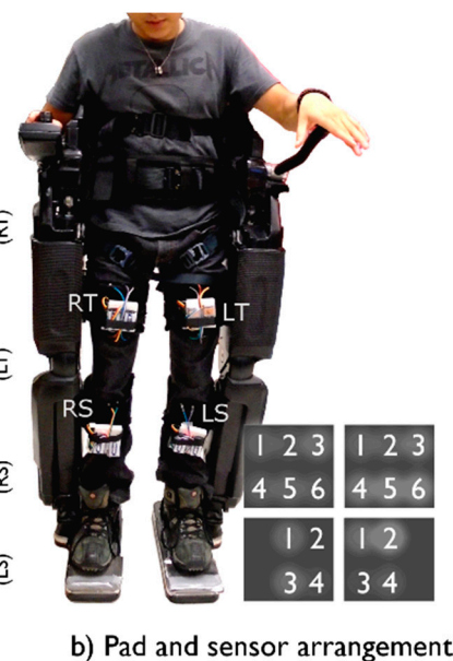
Figure 4. Pressure measurements of one SCI subject performing locomotion and non-locomotion tasks using a powered exoskeleton. (a) Twenty sensors arranged in 4 measuring pads (RT, RS, LT, LS). One trial including “stand up”, “walk”, “turn right”, “turn left” and “sit down” tasks. LT sensors 5 and 6 consistently show greater pressure levels, suggesting the lower strap of the subject's left thigh was adjusted tighter with the outer part receiving more force; (b) Rehab Rex exoskeleton from Rex Bionics is shown. Six sensors are used on thigh pads; 4 on shin pads. Shin sensors are positioned over risk areas caused by bony prominences corresponding to the tibia.
