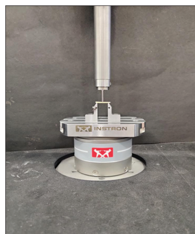
Figure 2: Determination of maximum force with INSTRON E3000 UTM (Electroplus). UTM: Universal Testing Machine
