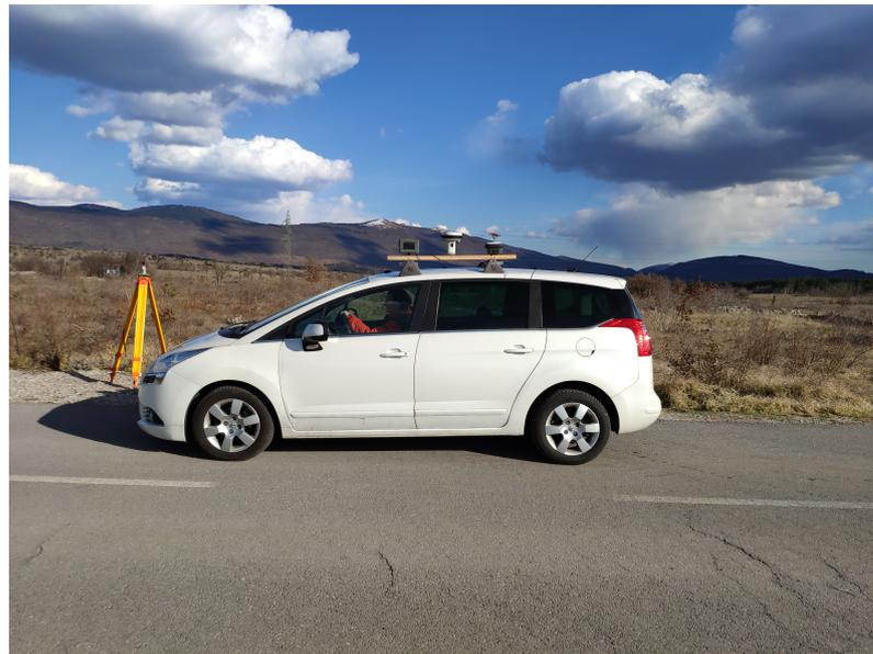
**Figure 3.** Vehicle with the GNSS receivers on the roof passing by the road static jammer (own study).
