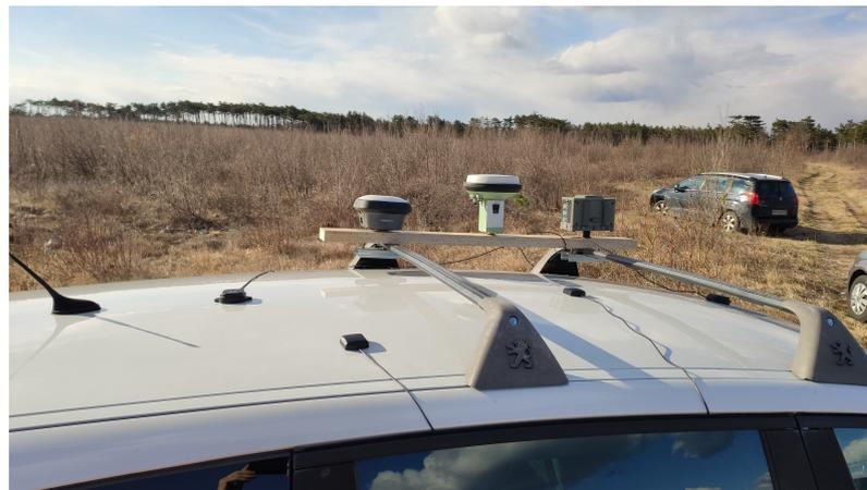
**Figure 1.** GNSS receivers set up on the roof of the vehicle (own study).
