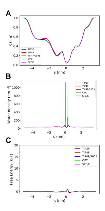
Figure S7: Profiles for the NNN mutant channel as a function of water model:  $\bf A$  radius,  $\bf B$  water density,  $\bf C$  water free energy.
