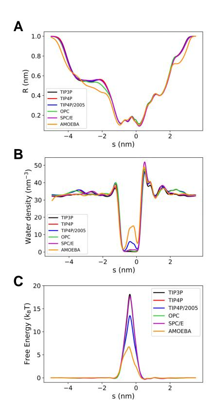
Figure S2: Profiles for the wild-type channel as a function of water model:  $\bf A$  radius,  $\bf B$  water density,  $\bf C$  water free energy.
