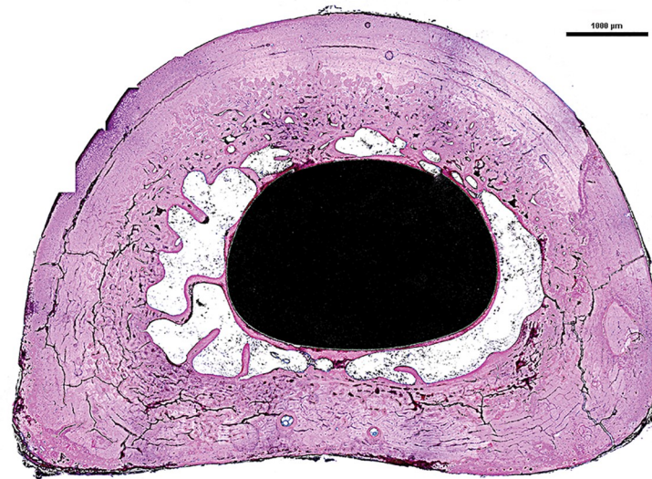
Fig 7. Photomicrograph of representative bone-endoprosthesis stem interface stained with Sanderson rapid bone stain: Black = endoprosthesis, pink = bone and blue = fibrous tissue. Scale bar = 1000 \mu m.
