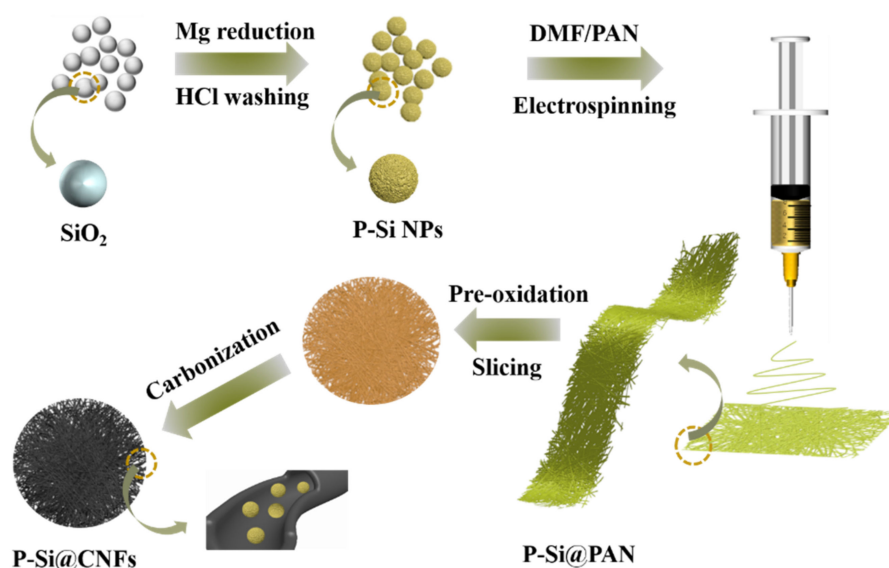
Scheme 1. Schematic diagram of the synthesis mechanism of the P–Si@CNF anode.
