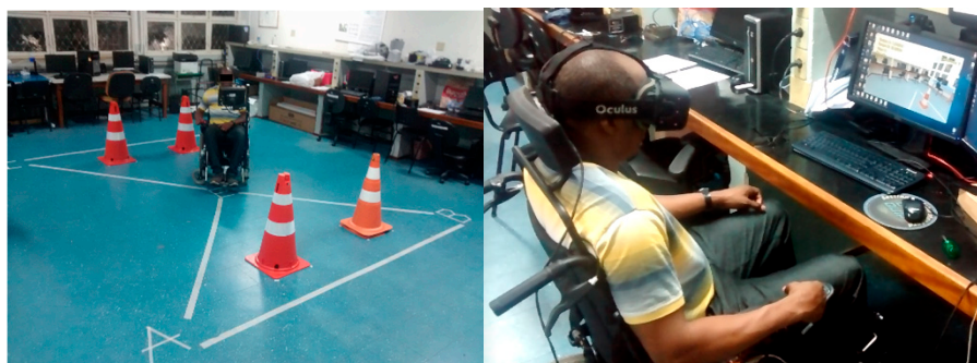
Figure 1. Participant testing the real EPW (left) and the virtual one (with the joystick as input interface) in the Simcadrom (right).
