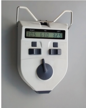
FIGURE 1: Digital pupillometer that shows in the center the ID and to the sides the NPD of each eye.
