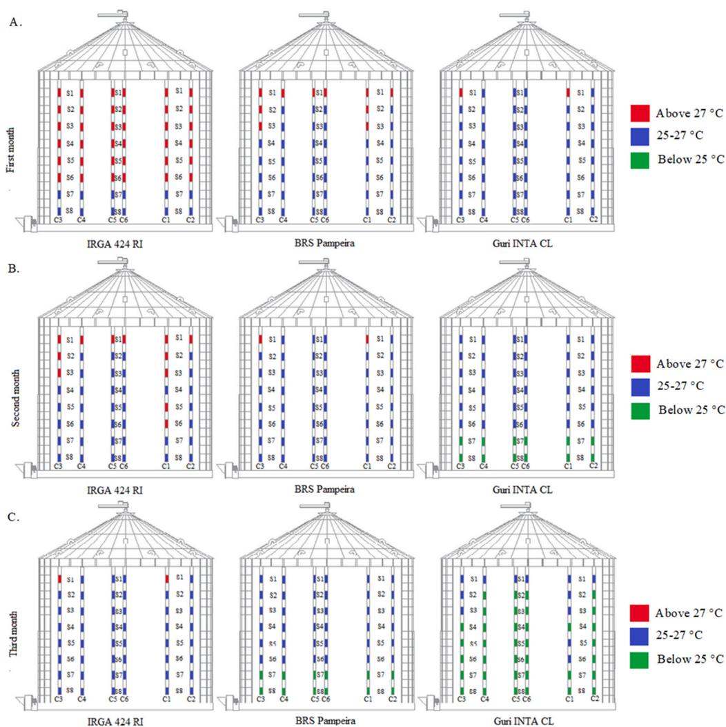
**Fig. 3.** Mean intergranular temperatures of the rice grain mass of the cultivars IRGA 424, BRS Pampeira, and Guri INTA evaluated in the lower and upper layers of the grain column in the silo-dryer-aerator: (A) first month, (B) second month, (C) third month.
