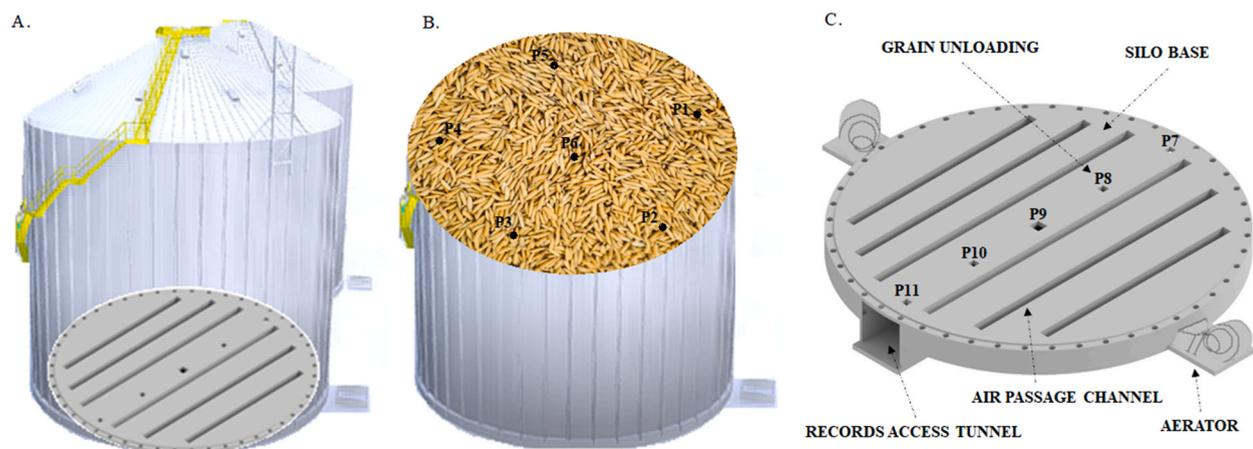
**Fig. 1.** (A) Structure of the silos dryer-aerator, (B) sampling points in the upper layers (position of the thermometric cables), (C) base structure of the silos-dryers-aerators, exhausters, ducts for air passage, discharge points, and sampling points of grains in the lower layers.
