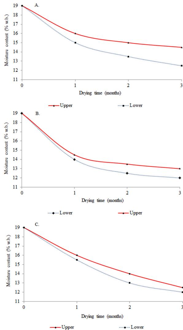
**Fig. 2.** Drying curves of rice grains (A) IRGA 424, (B) BRS Pampeira, (C) Guri INTA, evaluated in the lower and upper layers of the grain column in the silo-dryer-aerator, over 3 months of storage.
