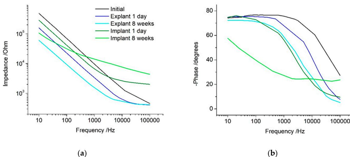
**Figure 5.** (a) Impedance; (b) Phase Angle. Electrochemical impedance spectroscopy of a platinum cochlear implant electrode at 0 V with an AC amplitude of 10 mV before cyclic voltammetry. Electrode initially tested in saline, implanted in a cochlea for 1 day, explanted after 1 day, reimplanted in cochlea for 8 weeks, and explanted after 8 weeks.
