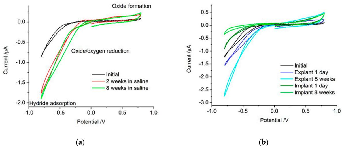
**Figure 1.** Voltammetric cycle of a platinum cochlear implant electrode from  $0 \rightarrow -0.8 \rightarrow 0.8 \rightarrow 0$  V at a scan rate of  $20 \text{ mV s}^{-1}$ : (a) electrode tested and stored in saline over 8 weeks and (b) electrode initially tested in saline, implanted in a cochlea for 1 day, explanted after 1 day, reimplanted in cochlea for 8 weeks, and explanted after 8 weeks.
