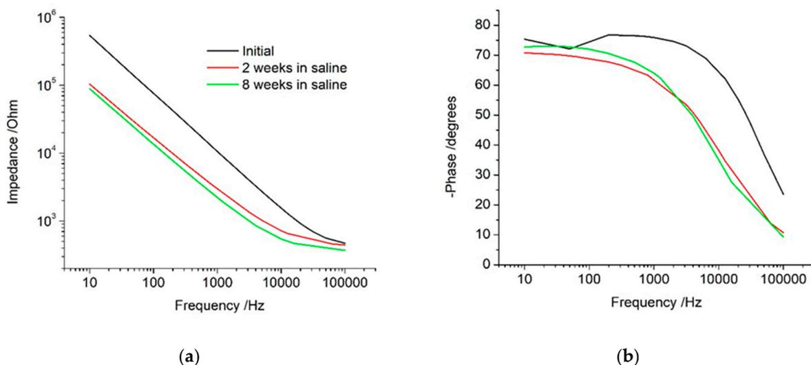
**Figure 2.** (a) Impedance; (b) Phase Angle. Electrochemical impedance spectroscopy of a platinum cochlear implant electrode at 0 V with an AC amplitude of 10 mV before cyclic voltammetry. Electrode tested and stored in saline over 8 weeks.
