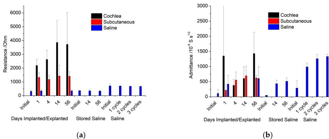
**Figure 4.** Equivalent circuit parameters (a) resistance and (b) admittance over time; initial, explanted, or stored electrode response in saline, or in vivo response in the cochlea or subcutaneously.
