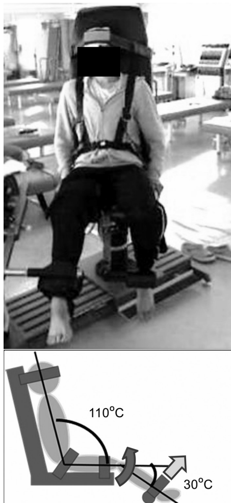
Fig. 3 . Posture for measuring knee extension force using the Cybex. The participant is placed in the sitting position on a chair, with the thigh and trunk at an angle of 110 degrees (hip flexion 70 degrees), knee flexion 30 degrees, and ankle joint angle in the middle position, with arms crossed in front of the chest.
