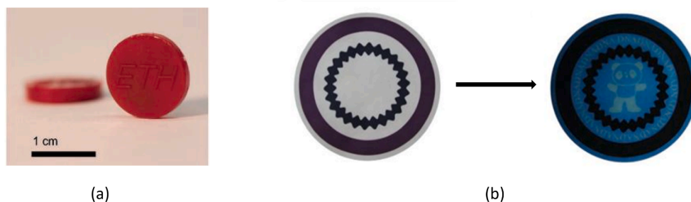
Fig. 3. (a) Polymers containing DNA sequences (Paunescu et al., 2013) and (b) invisible ink containing DNA for product authentication (Liu et al., 2017) (Printed with permission from Wiley and Royal Society of Chemistry).
