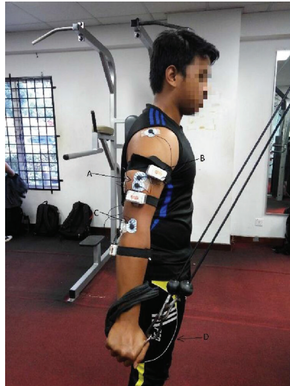
Figure 1. Subject performing an isometric contraction. A. Bipolar sEMG electrodes placed on the lateral head of the TB. B. Shimmer device, which wirelessly transmits sEMG signals to a computer. C. Reference electrode. D. Dominant hand holding the load.
