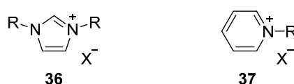
Figure 8. Generic structure of the two most investigated classes of ILCs: imidazolium (36) and pyridinium (37) salts. The imidazolium salts have the advantage that they allow easy asymmetric substitution at the heteroatoms of the ring.
