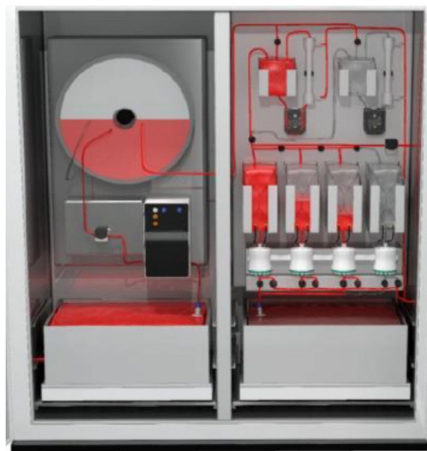
Fig. 2. Univercells' modular concept for combining USP and DSP in a small-footprint cabinet. The output from the high-productivity perfusion bioreactor (in the left chamber) is continuously feeding into the purification train (in the right chamber). The size and productivity of the perfusion bioreactor is matched with the downstream recovery process for efficient biologic manufacturing.
