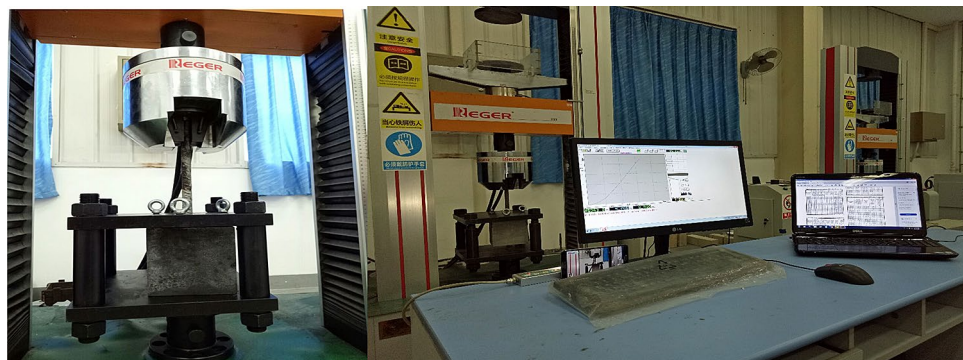
Figure 3. Pullout test lab and specimen installation 51 .
