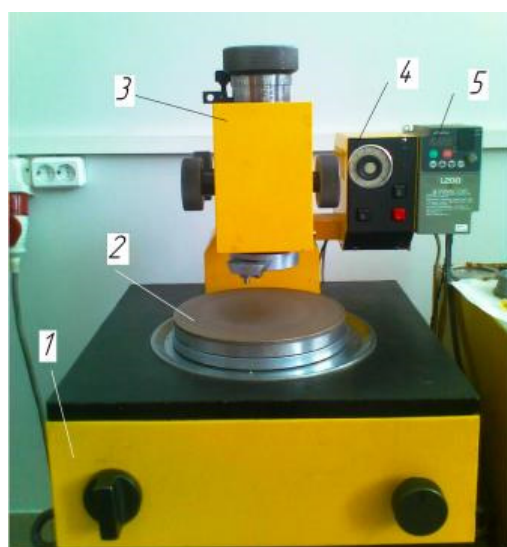
Figure 1. Lapping machine “Raster 220”. 1—drive unit, 2—Lapp, 3—pressure device, 4—control panel, 5—frequency converter.
