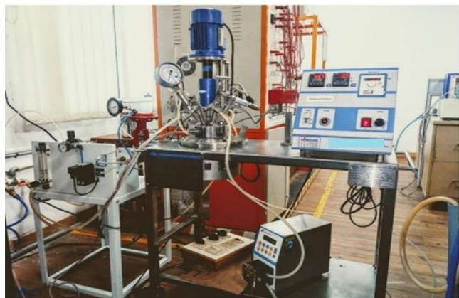
Figure 3. Lab-scale batch reactor in the Process Control Lab, MIT-Manipal.
