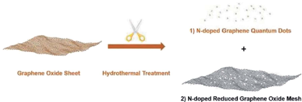
Fig. 7 Preparation of N-GQDs and N-RGO mesh. Reprinted with permission from ref. 194. Copyright 2018 John Wiley and Sons.
