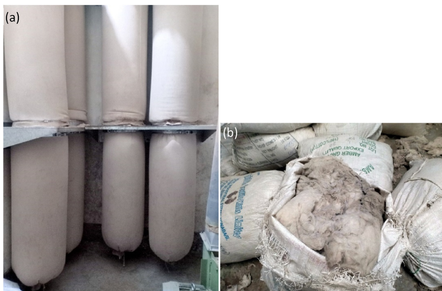
Figure 2. (a) Filter waste collector of humidification plant of the spinning mill, and (b) filter waste obtained from it.
