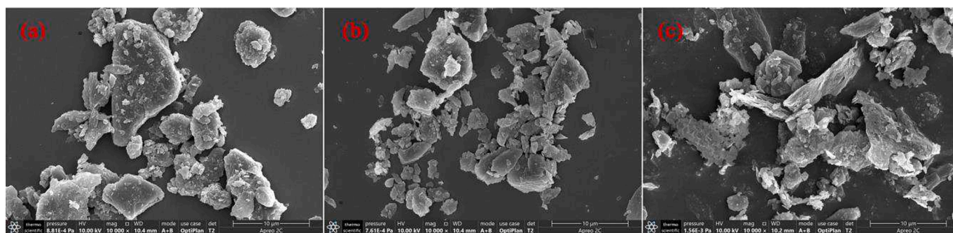
Fig. 11. SEM images of (a) raw ore, (b) CL concentrate (conventional leaching), and (c) UL concentrate (ultrasound leaching).
