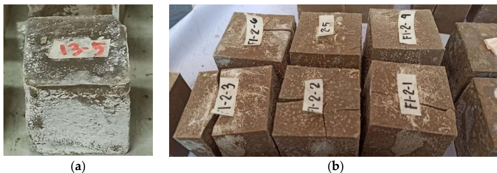
Figure 5. (a) Sample of a specimen that exhibits efflorescence. (b) Specimens that exhibit efflorescence and cracked before testing.
