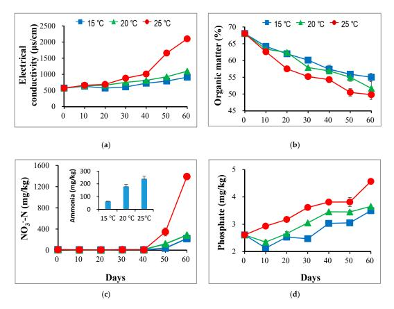
**Figure 1.** Changes of electrical conductivity (**a**), organic matter (**b**), ammonium, nitrate (**c**), and phosphate (**d**) levels during vermicomposting of sludge at 15 °C, 20 °C, and 25 °C, respectively.
