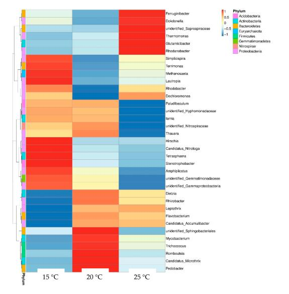
Figure 5. Heat map diagram of dominant bacteria for different sludge treatments at the genus level.
