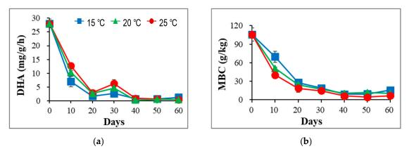
**Figure 2.** (**a**) Changes of dehydrogenase activity (DHA) and (**b**) microbial biomass carbon (MBC), during vermicomposting of sludge at 15 °C, 20 °C, and 25 °C, respectively.
