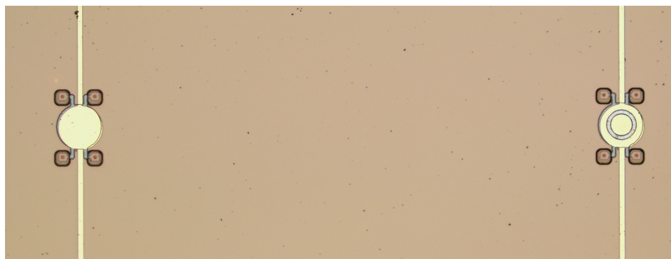
Figure 7. A uniform CMUT cell ( left ) and an embossed CMUT cell ( right ).
