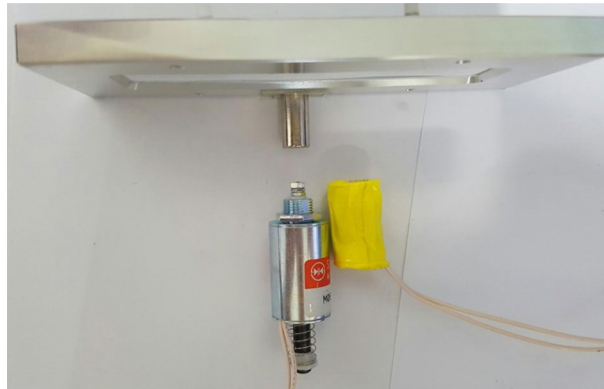
Fig. 3 Metal-plunger solenoid actuator and its solenoid coil
