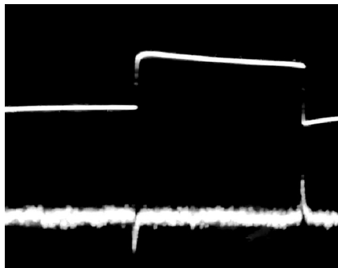
Figure 8. The upper beam is an acoustic signal in a 2 L container. The lower one is an electrical signal, which appears in the solution as the acoustic wave passes, recorded by silver chloride electrodes. The polarity of the electrical signal depends on the orientation of the electrodes relative to the acoustic radiator.
