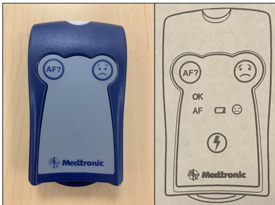
FIGURE 1 Model 2696 InCheck Patient Assistant device (9.6 × 5.6 × 2.2 cm). Left panel: photo of the physician assistant device. Right panel: diagram of physician assistant device with the symbols displayed for reference. Explanation of device buttons: “AF?”: The patient can press this button to query for atrial arrhythmia detection. If the device detects a median atrial rate for the last 12 beats that is faster than the set CL, then the “lightning bolt” button will light up. “Lightning bolt”: Pressing this button activates the TPARx application to temporarily allow ATP for 1:1 atrial tachycardia that satisfies all other criteria. “Sad face”: Pressing this button records symptoms without delivering ATP therapy. The device will display “OK” if there is no atrial tachycardia and “AF” if atrial tachycardia is detected [Color figure can be viewed at wileyonlinelibrary.com ]
