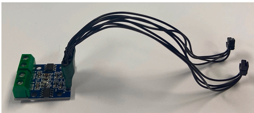
Fig. 8. Control to shutter driver board adapter.
